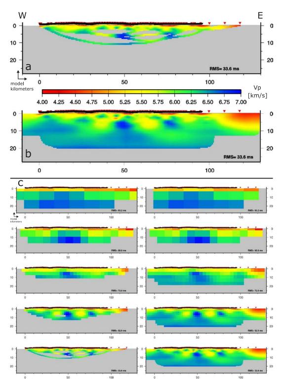
Figure 7.2.: Tomographic results of all available shots along the TIPTEQ profile (NVR/ESP/SH). Panel a shows the final image of the five inversion cycles, panel b shows the corresponding interpolated image. Part c of the figure shows the results of each of the five inversion cycles with decreasing cellsizes (cf. table 6.3). The velocity scale is valid for all tomographic images of that figure.
