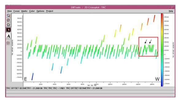
**Figure 3.10.:** DBTools 2–D Crossplot of all traces versus trace offset. The red box and the arrows point to the 3 shots with the wrong algebraic sign. The NVR and SH shots can be seen in green colors, other colors show ESP shots.
