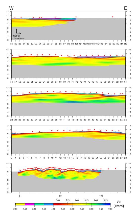
Figure F.14.: Final tomographic image without vertical exaggeration, lowermost panel shows total view, interpolated.
