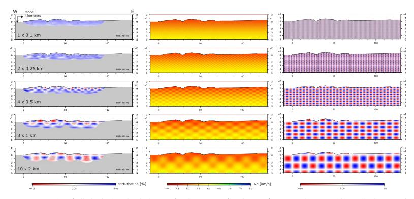
Figure F.2.: Results of all checkerboard calculations for the NVR + SH shot configuration shown together with the perturbated model and anomaly pattern.
