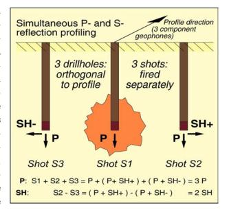
Figure 2.1.: Scheme of the Camouflet shooting method (Dohr, 1985) which uses a 3 hole setup (figure by M. Stiller, GFZ, pers. comm.).
