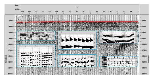
**Figure 6.1.:** The background image shows the flat onset of the first-breaks of FFID 1, because of the reduced travel-time (LMO). The insets show different characteristics of the first-breaks of shots along the profile, mainly of good quality. The inset in the lower right shows first-breaks more difficult to pick.
