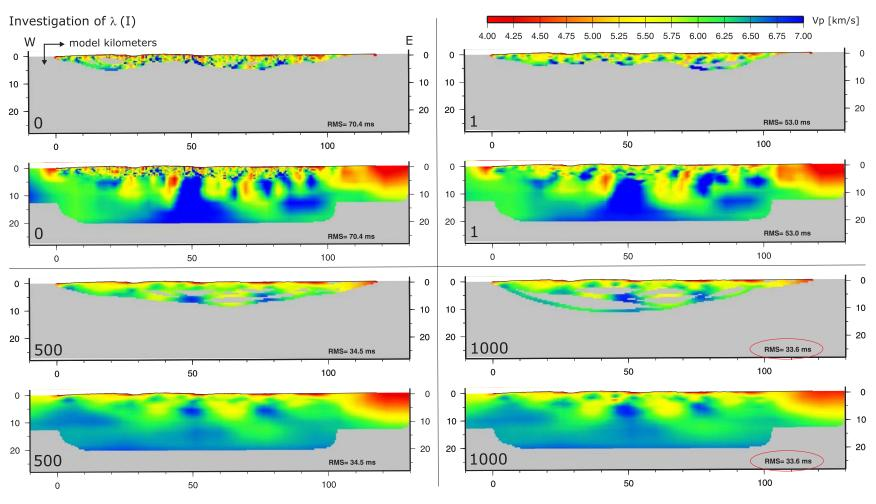
Figure E.3.: Investigation of  $\lambda$  using values of 0, 1, 500, and 1000, which turned out to be the best starting value for  $\lambda$ .
