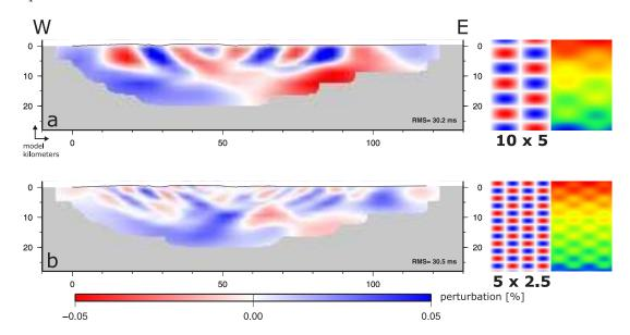
Figure 7.6.: Two checkerboard examples with anomalies of  $10 \times 5 \text{ km}$  (a) and  $5 \times 5.25 \text{ km}$  (b) in size, the anomaly pattern and perturbated velocity model are shown on the right. The elevation along profile is represented by the thin black line.
