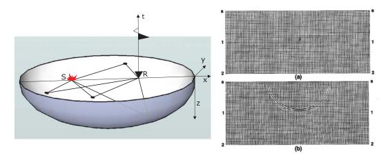
Figure 4.5.: Reflection surface ellipsoid of possible reflector locations with the same traveltime (left). Migration principle on smearing (right). (a) An unmigrated zero-offset section, consisting of a single non-zero sample on the central trace. (b) Migrated section, showing that the spike gets smeared onto the locus of possible reflection points – for this constant-velocity zero-offset 2-D example, a semicircle (Yilmaz, 2001).
