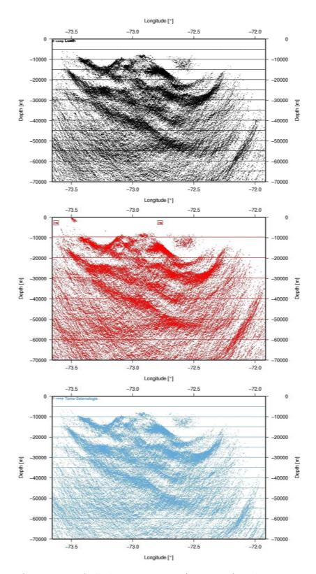
Figure 9.6.: Comparison of all three migrations (VE  $\approx$  1.5). The one using the SPOC velocity model is shown in black (top), the merged model in red (middle), and the seismology model in blue (bottom).
