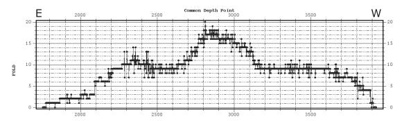
**Figure 3.9.:** 'XDB database display' plot of CDP versus fold of all 104 shots. The ESP shot configuration raises the fold in the central part of the profile from the nominal eightfold NVR configuration.
