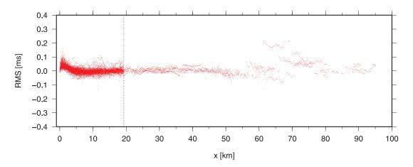
**Figure E.18.:** This figure shows again the differences between all picked and synthetic traveltimes for each receiver, this time plotted vs. all occurring offsets. The dashed line points to the maximal offset of 18 km for the standard shot NVR configuration.
