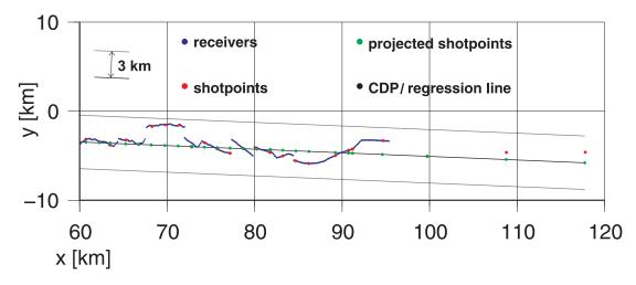
**Figure 6.2.:** Part of the receivers and shotpoints together with projected shotpoints and regression line (local coordinates). See appendix D for a map of the whole profile.
