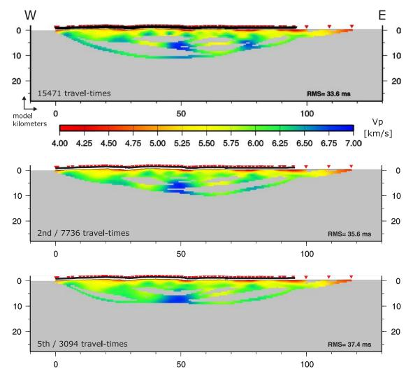
Figure 7.7.: Inversions with a reduced number of travel-times using every second (middle) and fifth line (lower) of the travel-time file in comparison to all travel-times (upper panel).
