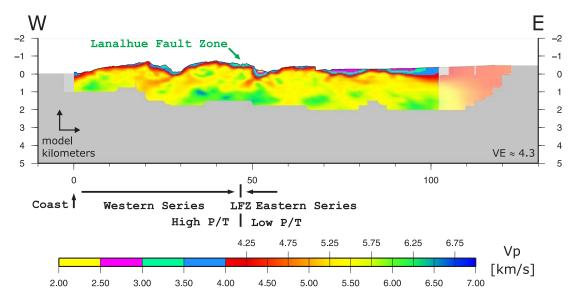
**Figure 10.14.:** Final tomographic image using NVR, SH shots and three shots off the line in the east. The sediment covered Central Valley starts at approximately x = 70 km.
