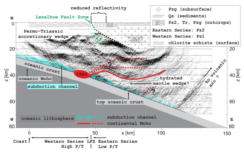
Figure 10.6.: Interpretation of the crustal structure and features at the plate interface for the TIPTEQ poststack depth migrated seismic section. The figure is modified after Groß, Micksch, and TIPTEQ Research Group (2008). See text for details and references.
