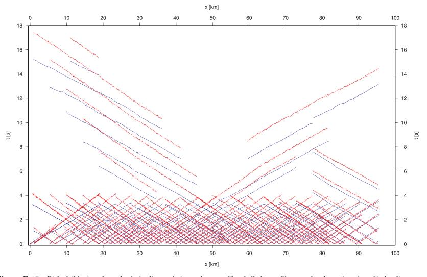
Figure E.15.: Picked (blue) and synthetic (red) travel-times along profile of all shots. Close to the shotpoints (t=0) the divergence between the calculated and picked travel-times seem to be admissible. Later than 2 s, the discrepancy increases rapidly up to  $\approx 1.5$  seconds for ESP shots (x=0 - 5 km, t=14 - 18 s), which can not be accepted.
