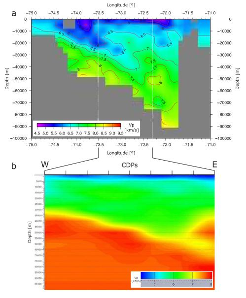
Figure 9.2.: Tomographic model at  $\approx 38.2^{\circ}$  S from seismology data (Haberland et al., 2008). Part b of the figure shows the ProMAX velocity model along the TIPTEQ transect. Confer figure 9.1d to compare differences in the velocity models).
