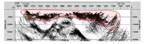
Figure 5.2.: The first kilometers of an example migration with airblast and first-break noise still contained in the data (red mask).
