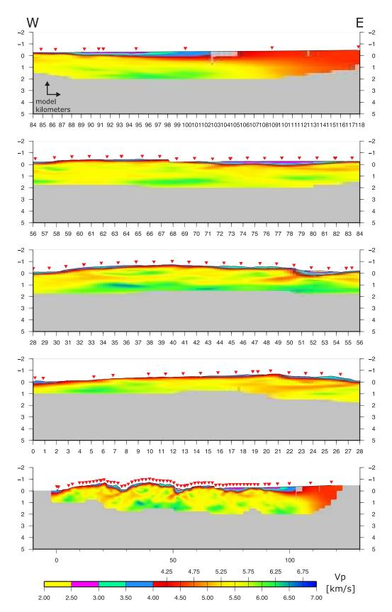
Figure F.16.: Final tomographic image without vertical exaggeration including shots off the line, lowermost panel shows total view, interpolated.
