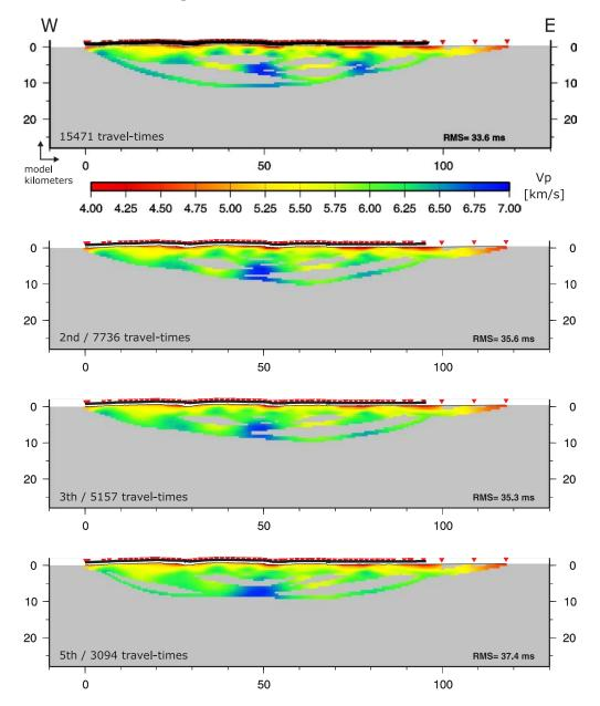
**Figure E.9.:** Inversions with a reduced number of travel-times using every second, third and fifth line of the travel-time file in comparison to all travel-times (upper panel).
