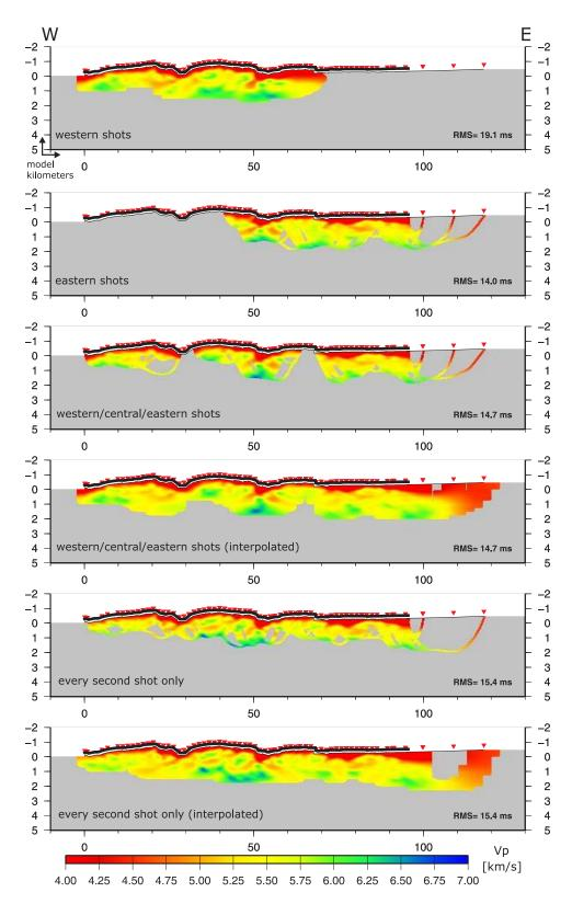
**Figure F.4.:** Variations in the number of NVR and SH shotpoints reproduce the observed structures and velocities using all NVR and SH shots. Notable differences occur in the central part of the profile (x = 40 - 50 km), where we observe very high velocities at the lower end of the profile.
