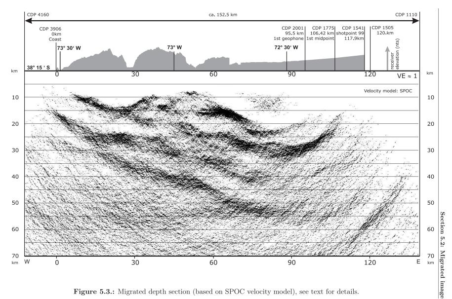
Figure 5.3.: Migrated depth section (based on SPOC velocity model), see text for details.
