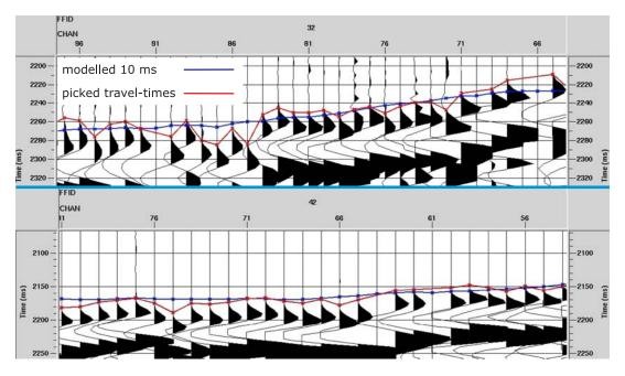
Figure 8.6.: Synthetic and picked travel-times together with shot data. The blue line belongs to the synthetic first-breaks with a pickerror of 10 ms, the red line shows picked travel-times. A very good fit is achieved, showing the quality of the inversion without the ESP shots. A comparison of the modeled travel-times calculated with both used shot configurations is provided in the appendix in figure F.11.
