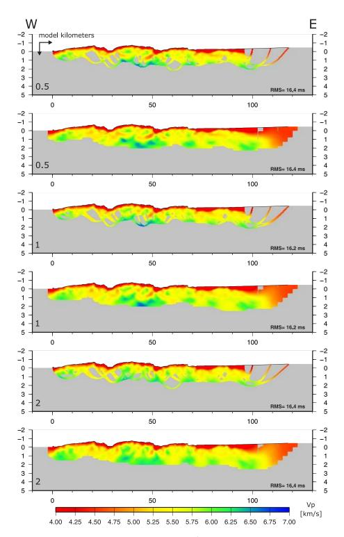
Figure F.12.: Horizontal vs. vertical smoothness/flatness investigation. A small  $s_z$  favors horizontal structures, whereas a large  $s_z$  leads to vertical structures. This trend is already visible in the small range of values for  $s_z$  used in the shown inversions. The RMS values lie between 16.2 to 16.4 ms. A value of 0.25 was used to obtain comparable results to the inversion with ESP shots, and provides a RMS value of 16.3 ms (cf. figure 8.2).
