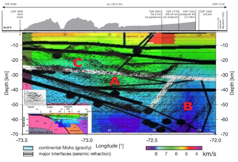
**Figure 10.13.:** This figure shows the seismic model underlain by the ISSA Vp tomographic velocity model and wide-angle velocity and density derived interfaces. A: Region of possibly hydrated/serpentinized mantle; B: Normal mantle; C: SPOC velocity model 7 km/s layer. Modified after Krawczyk et al. (2007), see text for more details.
