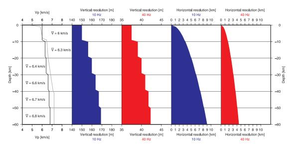
Figure 4.10.: Horizontal and vertical resolution up to a depth of 60 km for the TIPTEQ data set. The black line shows a mean crustal velocity recalculated every ten kilometers derived from a 1-D velocity depth function of the SPOC wide-angle velocity model (grey line). These mean velocities were used in the calculations shown in red and blue. The smooth curves of the horizontal resolution result from a depth dependency of the Fresnel zone (cf. equation 4.5).
