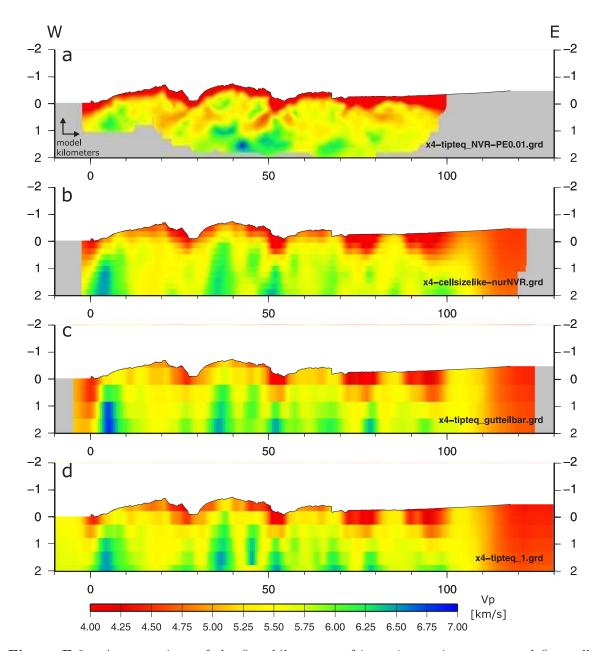
Figure F.8.: A comparison of the first kilometers of inversions using coarse and fine cells with different pickerrors. Results b - d belong to inversions including the ESP shots (z = -2 to 28 km), and use a pickerror of 0.03 s, whereas panel a uses 10 ms and lacks the ESP shots. The lower three images resemble each other remarkably well, and some features are even comparable with the fine-structured, low-pickerror inversion result shown in a.
