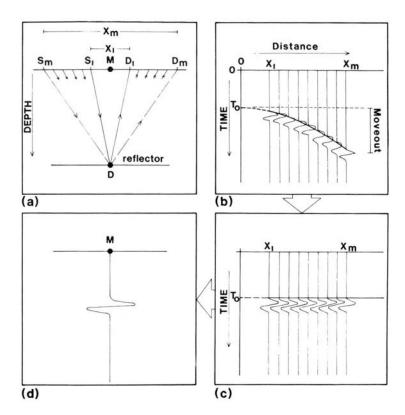
**Figure 4.4.:** The process and result of CDP sorting (a), NMO correction (b/c) and stacking (d) (Beaumont and Foster, 1989).
