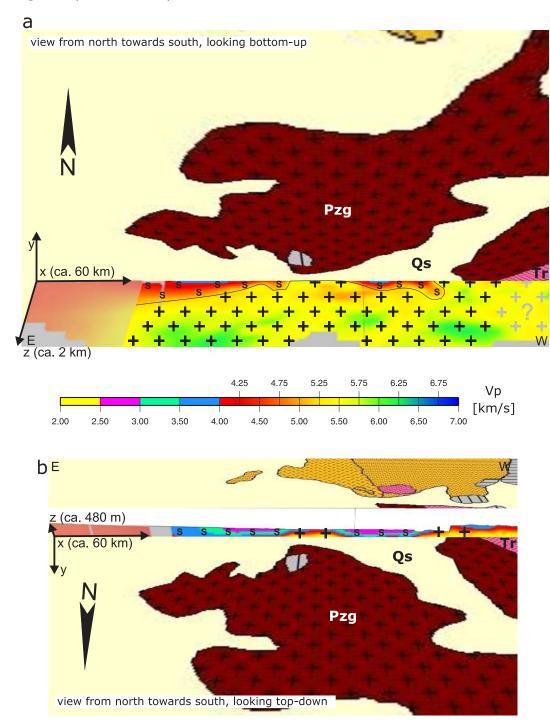
Figure 10.16.: This figure illustrates the subsurface continuation of the Coastal Batholith, Pzg (signature: +) and the Quaternary sediments, Qs (S). The thickness of the sediments reaches  $\approx 1$  km at the western border of the mask, which limits the confidence area.
