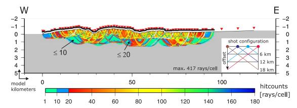
**Figure 8.3.:** Hitcounts for NVR and SH shots only. White colors account for hitcount values greater than 180. The inset on the right shows the four possible shot configurations, see text for more details.
