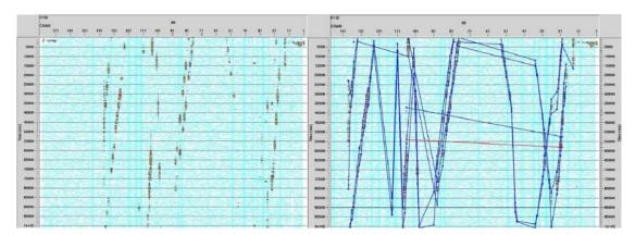
**Figure 3.4.:** The left side of this figure shows the unfiltered data of FFID 69, the colored streaks are the noise patterns produced by cars. Up to 4 surgical mutes are needed to cut out all disturbances (right).
