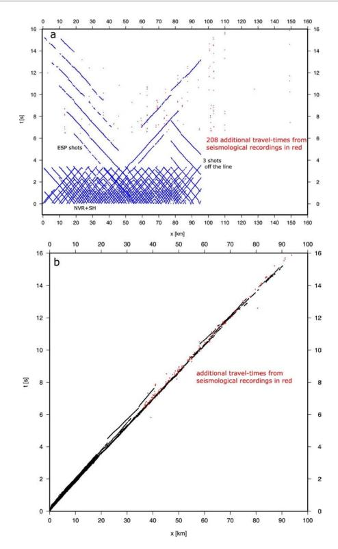
Figure 7.12.: All picked travel-times vs. profile kilometer (a) and travel-times vs. occurring offsets (b), including additional seismology picks (cf. figure 6.3 and 6.4). See text for details.
