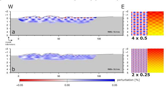
**Figure 8.5.:** Two checkerboard examples (NVR + SH shots) with anomalies of  $10 \times 5 \text{ km}$  and  $5 \times 5.25 \text{ km}$  in size, the anomaly pattern and perturbated velocity model is shown on the right.
