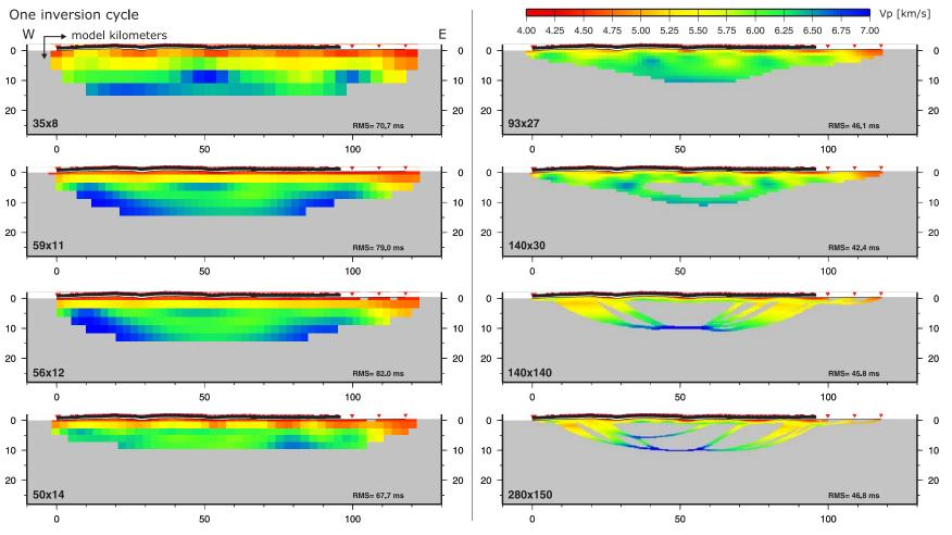
**Figure E.5.:** Results of one inversion cycle only with varying cellsizes. In shallow depths the results may be comparable to each other (< 3 km). Using only small cells, the rays of one shot tend to focus in one 'single beam' with unrealistic velocities (too smooth, too fast) along the travel path.
