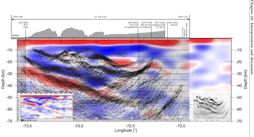
Figure 10.11.: Receiver functions and the poststack seismic image. Red colors show a velocity decrease, blue colors a velocity increase, respectively. See text for more details. The RF image and interpretation of the converters were kindly provided by Andreas Rietbrock (University of Liverpool, UK).
