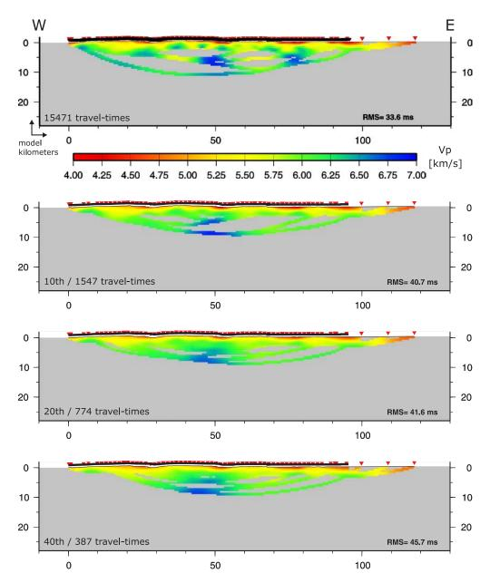
Figure E.10.: Inversions with a reduced number of travel-times using every tenth, twentieth and fortieth line of the travel-time file in comparison to all travel-times (upper panel).
