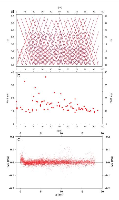
Figure F.10.: Figure F.10a shows the picked and calculated travel-times including a random pickerror of 10 ms. The two times match very closely. Part b shows the RMS error of each shot along profile which mainly lies between 10 and 20 ms. Panel c shows the RMS values of all receivers sorted after offset. A slight drop in point density can be observed for offsets greater than 12 kilometers, resulting from the shot/spread configuration (cf. figure 8.3).
