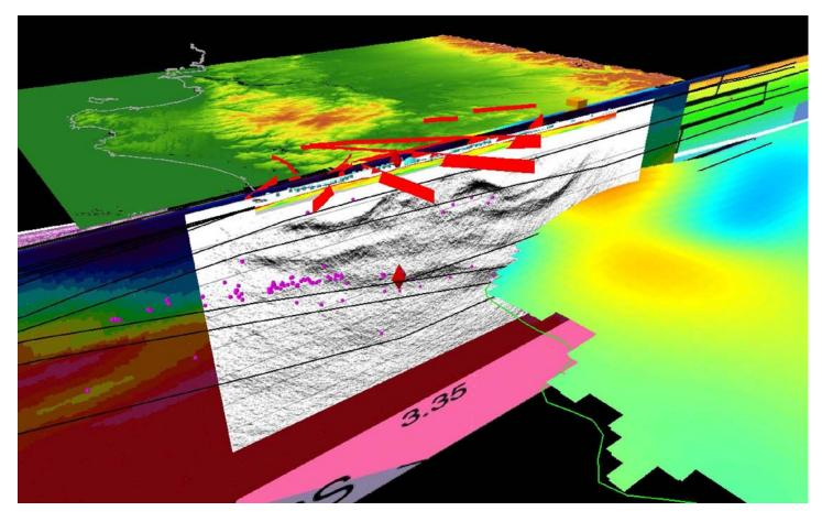
Figure H.2.: TIPTEQ related data visualized in Fledermaus. Besides the reflection seismic image in the center, tomographic velocity distributions, velocity and density interfaces, earthquake hypocenters, and digital elevations are shown.
