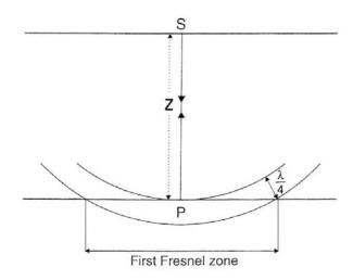
Figure 4.9.: Geometry of the Fresnel zone (Jones, 1999).
