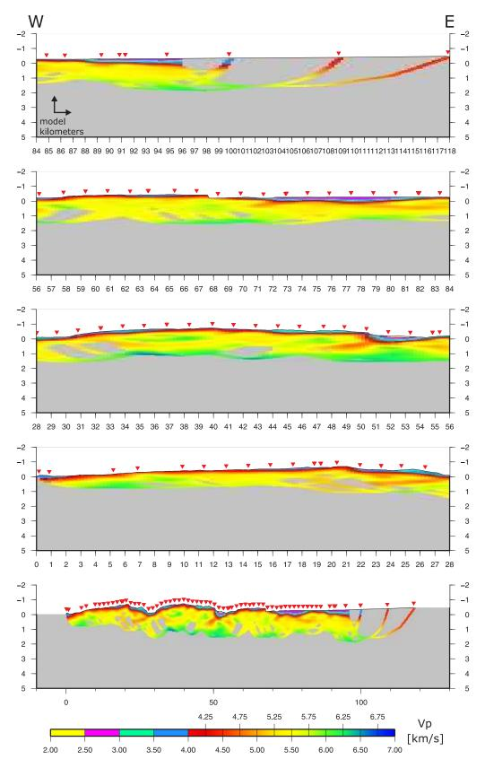
Figure F.15.: Final tomographic image without vertical exaggeration including shots off the line, lowermost panel shows total view.
