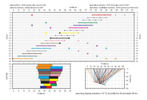
**Figure 2.3.:** ESP (colored) and NVR (black) shot and receiver configuration for each set-up day. Additional shots at certain offsets to the active spread focus on the plate interface at a depth of 38 km. The lower part of the figure shows the resulting CDP fold and ray-paths of the ESP shots (figure by M. Stiller, GFZ, pers. comm.).
