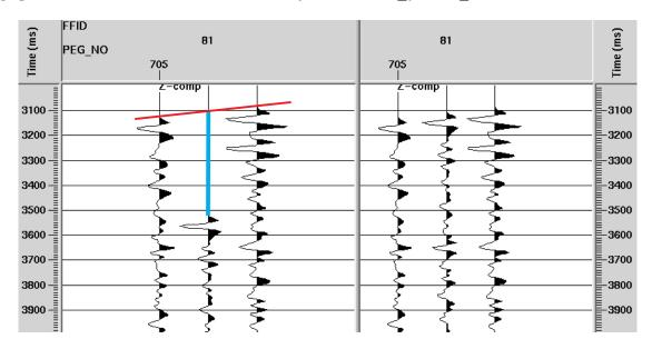
Figure 3.1.: The mean first-break time calculated from neighboring traces gives the new first-break time (red line). The blue line marks the time the trace needs to be shifted.
