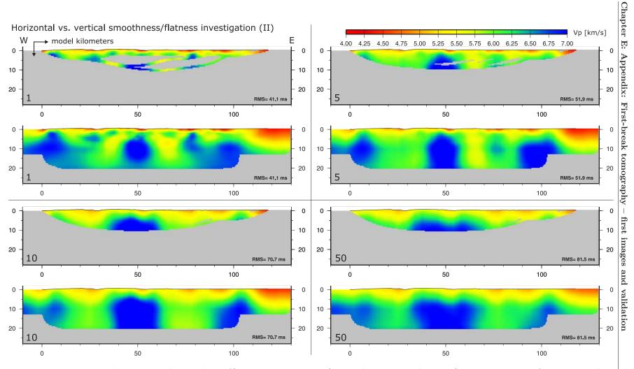
Figure E.2.: Horizontal vs. vertical smoothness/flatness investigation (ray and interpolated images) using  $s_z$  values of 1, 5, 10, and 50.
