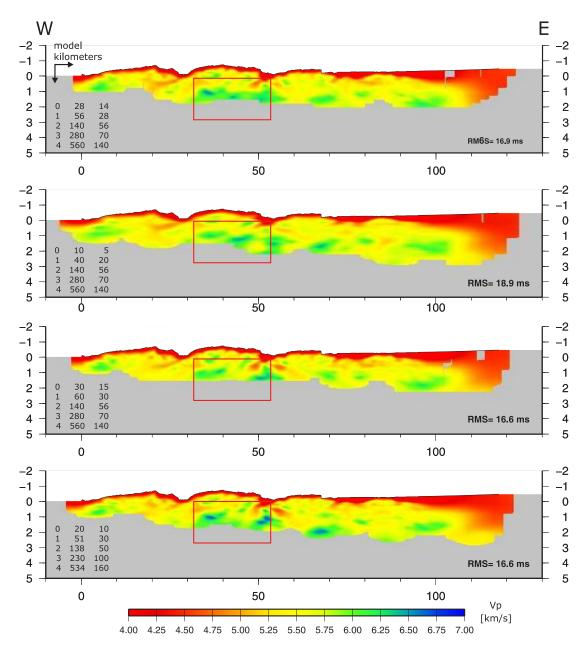
Figure F.6.: Effects produced by variations in the inversion cellsizes can also be observed in the inversion with the NVR + SH shots only, but of a lower magnitude. Major differences are marked by a red box in the central part of the profile.
