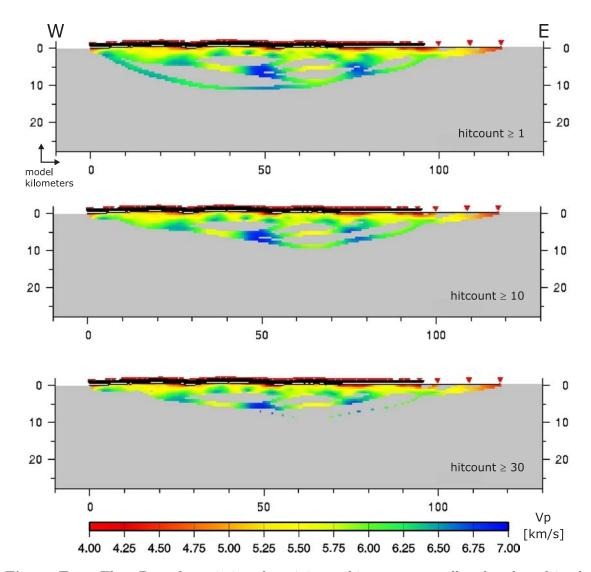
**Figure E.8.:** The effect of restricting the minimum hitcounts per cell to be plotted in the resulting velocity model is shown in this figure. The upper panel uses every cell at least one ray has passed through. The panel in the middle uses only cells with a hitcount of 10 and higher, the lower panel uses cells with hitcounts greater than 30.
