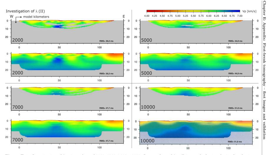
Figure E.4.: Investigation of  $\lambda$  using values of 2000, 5000, 7000, 10000. Large values of  $\lambda$  still image the basic velocity distribution quite well.
