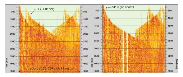
Figure 3.11.: Two test stacks one with (left) and one without FFID 99 (right) demonstrate the correct alignment of the shot with the suspicious offset values in the ProMAX database.
