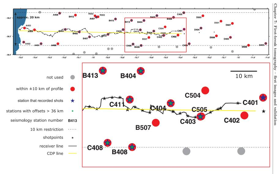
Figure 7.11.: Distribution of the used seismology stations along the TIPTEQ profile with labels for each exclusion criteria.
