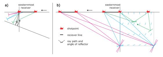
**Figure 5.4.:** Preferred imaging of steep dips at the ends of the profile.
