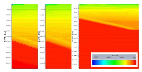
Figure 4.2.: Part of the SPOC input model is shown on the left panel, the corresponding smoothed model is shown in the middle. The right panel shows the complete smoothed and extended model used for migration.
