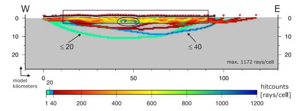
**Figure 7.4.:** Plot of the hitcounts for the inversion using all available shots. The black rectangle outlines the area with a hitcount value between 300 and 800, the hitcount maxima with 1172 counts is marked by an ellipse.
