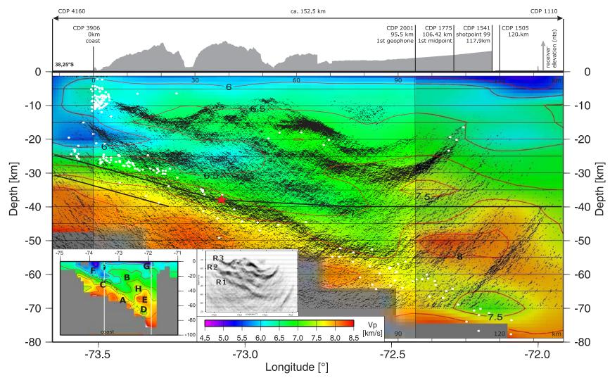
Figure 10.9.: TIPTEQ poststack section overlain on the velocity model derived from the inversion of seismological travel-times of local seismicity and shots from the active source experiment. See text for more details. The velocity data were kindly provided by Christian Haberland (University of Potsdam/GFZ).
