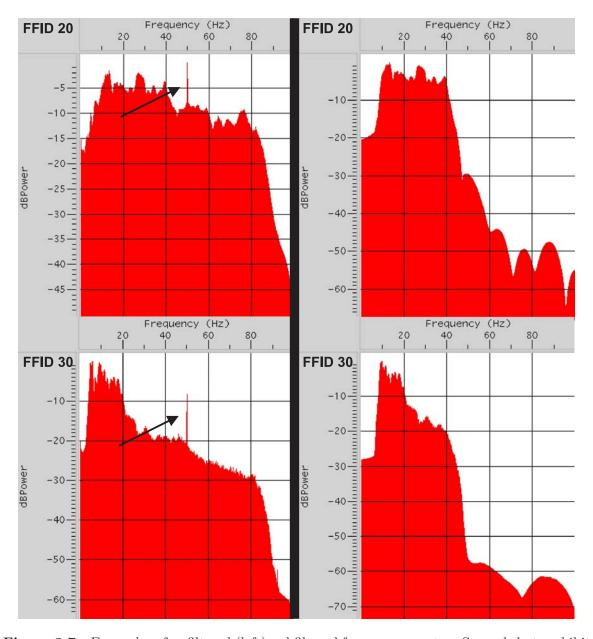
**Figure 3.7.:** Examples of unfiltered (left)and filtered frequency spectra. Several shots exhibit a distinct maximum at 50 Hz which is the typical alternating frequency for electrical AC currents (arrows in figure) inducing this frequency in the cables of the geophone. The right part of the figure shows the effect of the finally chosen Ormsby bandpass filter with corner frequencies of 6 - 10 - 35 - 50 Hz.
