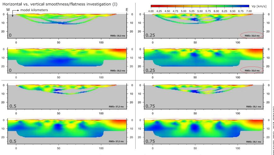
Figure E.1.: Horizontal vs. vertical smoothness/flatness investigation (ray and interpolated images) using  $s_z$  values of 0, 0.25, 0.5, and 0.75. The red ellipse marks the RMS value of the best fitting model. Shotpoint and receiver locations are not shown, the elevation along profile is represented by the thin black line.
