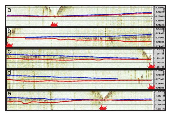
**Figure 3.3.:** Representative airblast mutes for five TIPTEQ shots. Almost no airblast disturbance (a), a gradually widening mute to greater offsets (b/c) or the widening starts at a certain offset (d/e). Shotpoints are marked with red symbols along the whole active spread of 18 km, the length of the time window is  $\approx 4$  s.
