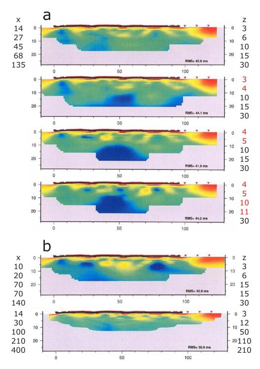
**Figure 7.15.:** Variation of the inversion cellsizes, part II. Panel a of the figure compares small changes in the number off cells in z-direction. The cellnumbers in x-direction are kept fixed. Part b shows the effect of rapidly increasing cellnumbers.
