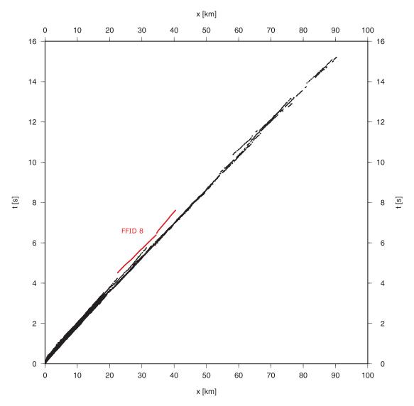
Figure 6.4.: All picked travel-times vs. occurring offsets.
