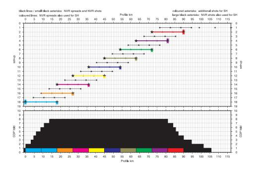
Figure 2.2.: The NVR (black) and SH (colored) shot and receiver configuration is plotted along profile kilometer for each spread set-up. The first active receiver spread starts at  $\approx$  95 km. The lower part of the figure shows the corresponding CDP fold (figure by M. Stiller, GFZ, pers. comm.).
