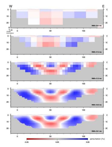
**Figure E.11.:** All five inversion cycles for a checker board calculation with a perturbation anomaly size of  $20 \times 10$  km.
