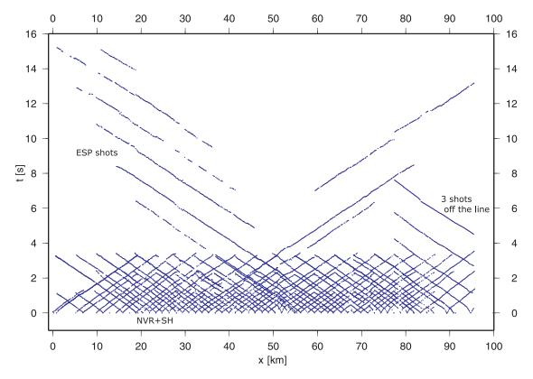
Figure 6.3.: All picked travel-times vs. profile kilometer.
