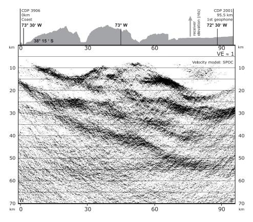
Figure 5.5.: Depth migrated section covering only the extend of the receiver line.
