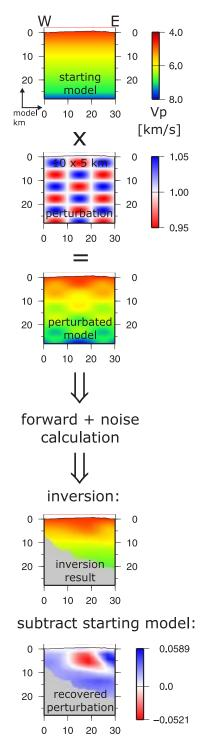
Figure 7.5.: Checkerboard calculation workflow.
