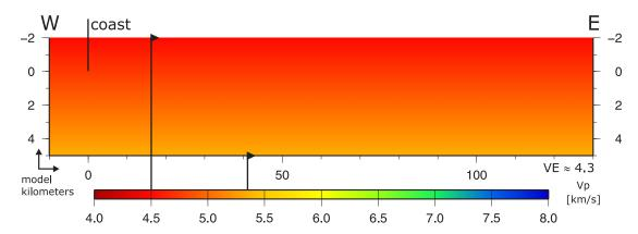
**Figure 8.1.:** Model setup and starting velocity model used for the inversion of the NVR + SH shots only. The velocities range from 4.5 - 5.375 km/s.
