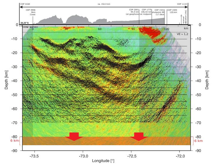
Figure H.4.: Illustration of the stretched KPSDM and poststack image. The lower end of the KPSDM image (z = 80 km) is stretched to z = 86 km depth, resulting in a stretch factor of 1.075. Of course, the poststack image can be bulged upwards the same amount to fit both sections.
