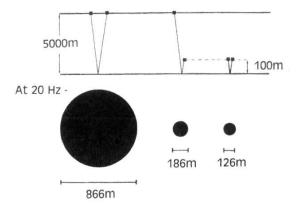
**Figure 4.11.:** Approach to minimize Fresnel zones. The black circles demonstrate the relative size of the Fresnel zone for different marine source/receiver configurations at the surface and using a deep-towed source and/or receiver (cf. equation 4.5). For the speed of sound in water a velocity of 1.5 km/s was used, the source frequency is 20 Hz (Jones, 1999).
