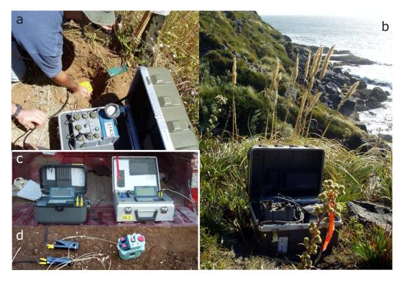
Figure 2.4.: Receiver stations and shooting equipment. Panel a shows the buried and oriented 3-component geophone and the EDL recording unit in a weatherproof box. The picturesque last receiver station 955 at the Pacific Ocean is shown in b. Panel c shows two similar boxes to record the exact shot times, e.g., with pliers around the ignition lead, not yet connected to the trigger box (d). Image courtesy of C. Krawcyzk.
