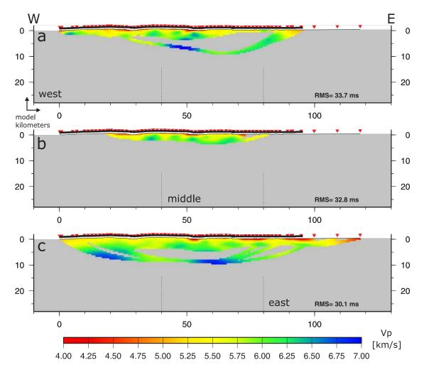
**Figure 7.8.:** Inversion results using a reduced number of shotpoints. In panel a, only the western third of shots is used (including ESP shots along the whole profile), panel b presents the result using only the middle part of the shots, c shows the resultant inversion image using only the eastern third of shotpoints.
