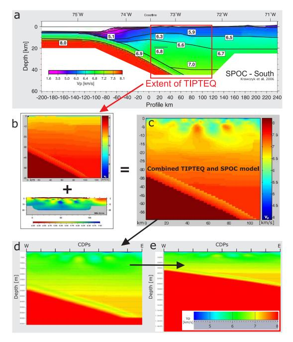
**Figure 9.1.:** The SPOC model (a) was imported into MATLAB and merged with the interpolated tomographic model calculated from all shots (NVR/SH/ESP; b/c). The CDPs were assigned to the resultant velocity model, to be able to import it into ProMAX. There, it was further altered and smoothed to cope with steps in velocity and model size (d/e).
