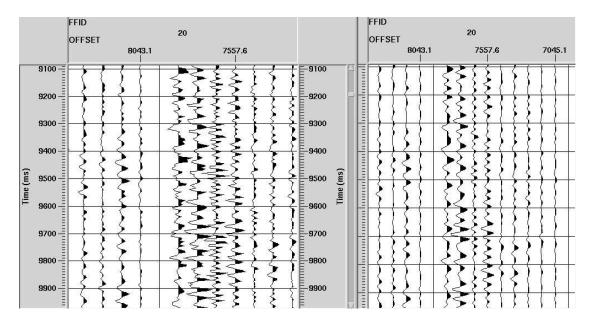
Figure 3.8.: Data example of unfiltered (left) and filtered data (right) of FFID 20, where we can observe a lack of high frequencies in the traces.
