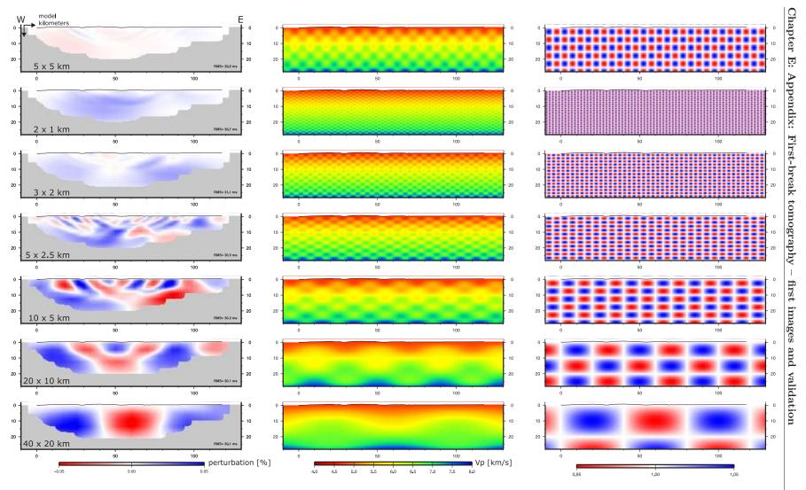
Figure E.12.: Results of all conducted checkerboard tests together with the corresponding perturbated models the synthetic travel-times were calculated with, and the used perturbation pattern.
