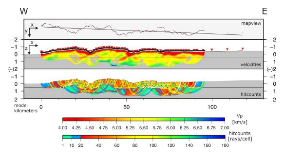
Figure 8.4.: A direct comparison of the geometry, velocity model, and hitcount results.
