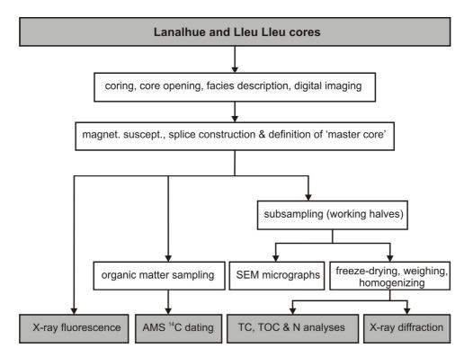
Figure 1.7 Operation chart for the lacustrine sediment records of Lago Lanalhue and Lago Lleu Lleu
