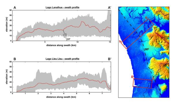
**Figure 3.9:** Topographic swath profiles across the Lanalhue and Lleu Lleu swells. Right: Areas of the profiles (A-A': Lanalhue swell. B-B': Lleu Lleu swell). Left: Lanalhue profile (A-A') and Lleu Lleu profile (B-B'). Each profile shows maximum, minimum (shading), and mean elevations (red solid line) of topography. MF = Morguilla Fault.
