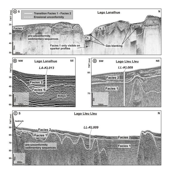
**Figure 3.5:** Seismic profiles of Lago Lanalhue and Lago Lleu Lleu. The position of the respective seismic lines is indicated in Figure 3.4 (a+b). The unconformity, stratigraphic boundary, and core-to-seismic correlation are shown. A: S-N pinger profile in the central part of Lago Lanalhue. B: NW-SE sparker profile with projection of LA-KL013. C: S-N sparker profile in the central part of Lago Lleu Lleu with projection of LL-KL009. D: Pinger profile with projection of LL-KL009.
