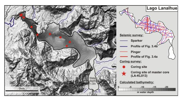
*Figure 3.4a:* Bathymetry, coring positions, and seismic survey lines of Lago Lanalhue. Bathymetry calculated using seismic profiles; isobath every 1 m.
