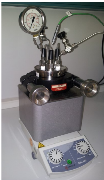
Figure 1: Laboratory autoclave setup including (from bottom to top) heater/stirrer, stainless steel autoclave in thermal insulating sheath, clamp, autoclave lid with electrodes, manometer and inlets for gas feed, liquid injection and temperature sensor.
