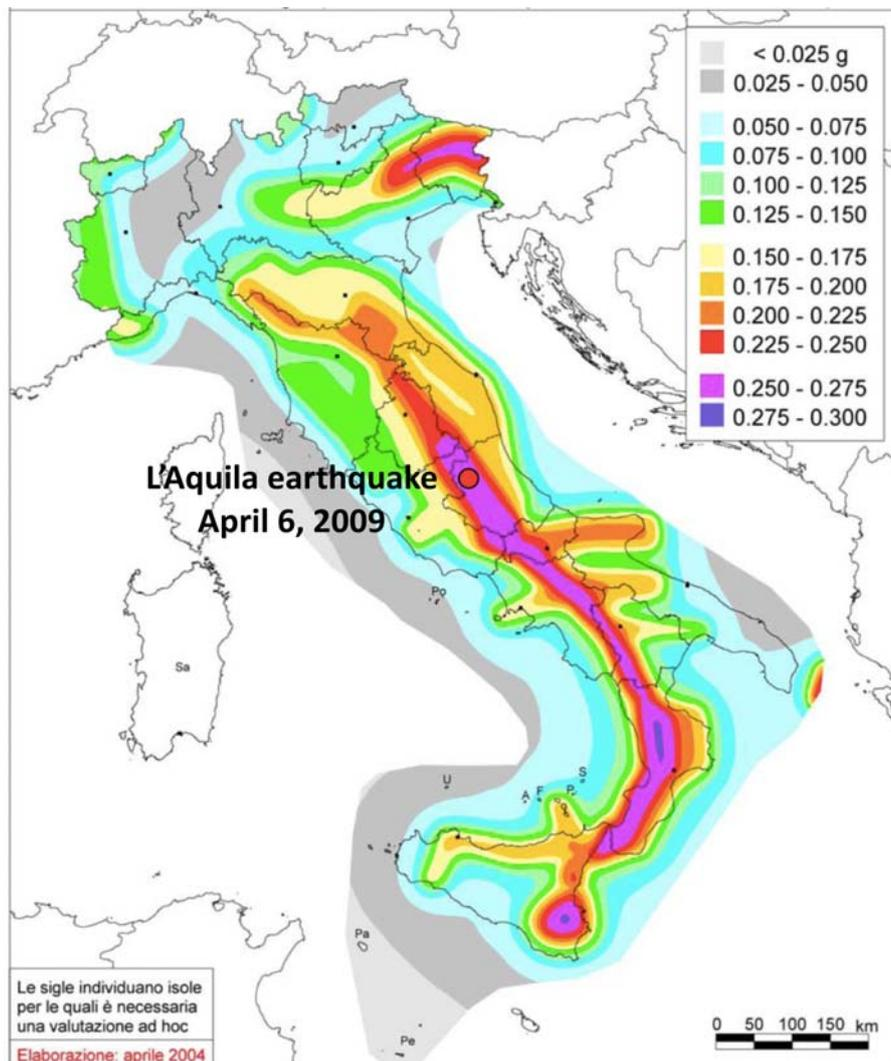
**Figure 1.2.** The probabilistic seismic hazard map for Italy [1], showing the location of the L'Aquila earthquake of 6 April 2009. The colors indicate the ground acceleration with a 10% probability of exceedance in 50 years, measured in units of surface gravitational acceleration,  $g = 9.8 \text{ m/s}^2$ .
