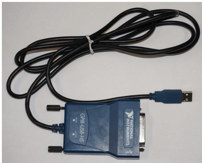
**Figure 54: USB to GPIB (IEEE-488) adapter from National Instruments**
