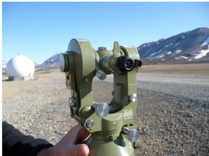
Figure 48: Theodolite used for determination of local antenna horizon masking
