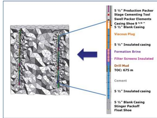
Fig. 9 Implementation of the well completion scheme into the inversion of the crosshole geoelectric field data.
