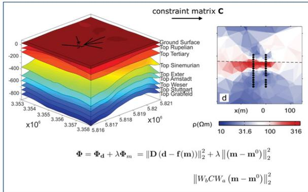
Fig. 8 Optimized imaging of the CO<sub>2</sub> signature in the reservoir zone: (a) Implementation of structural information [14] based on 3D seismic results as *a priori* constraint into the inversion of the surface-downhole geoelectric data [9].
