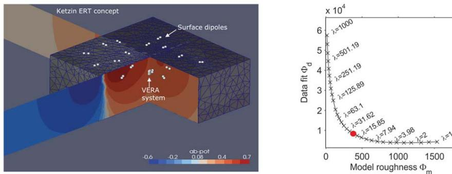
Fig. 6 Left hand: Visualization of the tomographic cube (side length 5 km, height 2 km) for the Ketzin case by means of unstructured tetrahedral elements. Right hand: The plot compares data misfit and model misfit as a function of spatial regularization [5].
