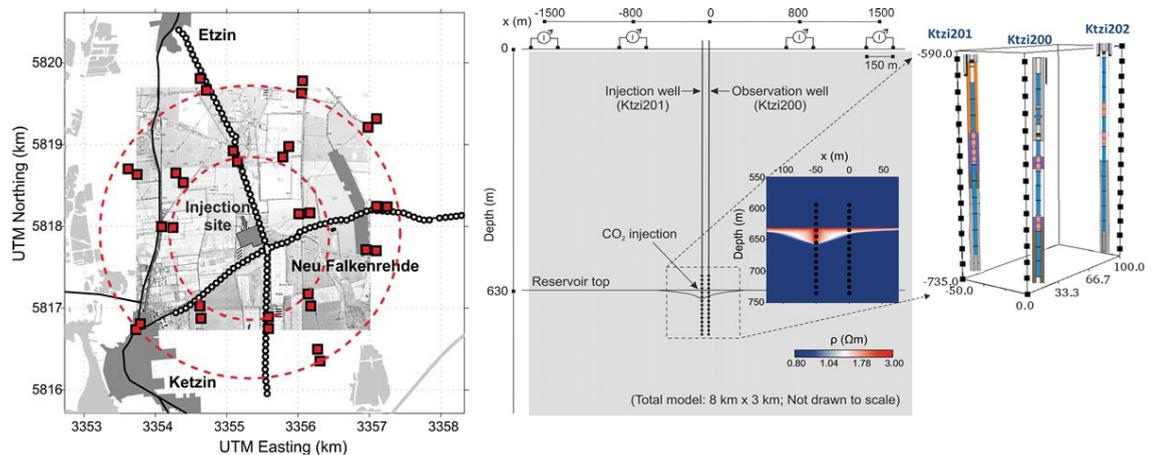
Fig. 1 Left hand: Area of the Ketzin test site, indicated by a white star. Pairs of red boxes mark the positions of the 16 non-permanent surface dipoles, each with a length of 150 m, as used for the periodical surface-downhole ERT (SD-ERT) surveys. Right hand: Schematic of the boreholes and the permanent VERA electrodes (black dots in dashed box). The rightmost illustration shows that the completions of the three Ketzin wells are different among each other.
