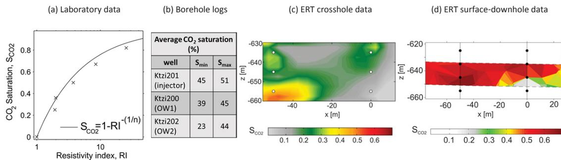
Fig. 7 Comparison of saturation results from different measurement methods: (a) laboratory data of Ketzin reservoir sandstone samples [11]; (b) borehole data of the Pulsed-Neutron-Gamma logs [12]; (c) saturation calculation for the crosshole ERT data, and (d) for the surface-downhole ERT data [5].
