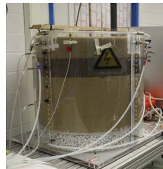
Fig. 11 Sandbox facility for studying salinization scenarios. The diameter of the cylinder is about 0.6 m. The fluid injection into the tank was realized by a peristaltic pump. A miniaturized electrode layout consisting of horizontal and vertical electrode strings has been developed [16].
