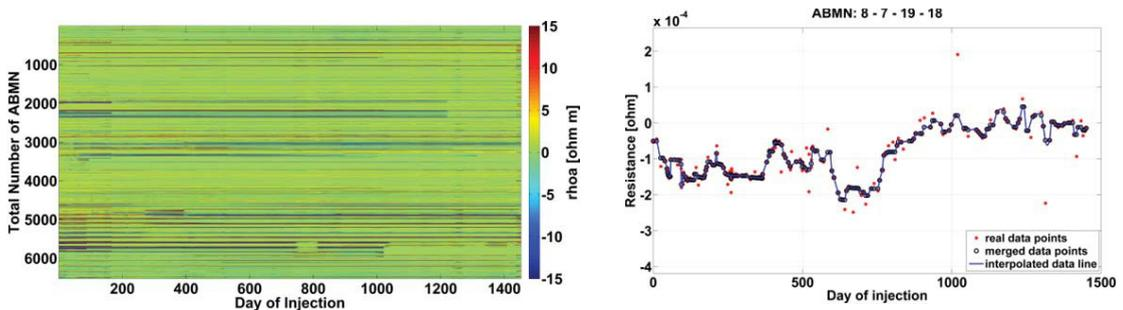
Fig. 5 Left hand: Automated archiving of the total number of 6590 deployed ABMN configurations in the crosshole ERT mode (apparent resistivity  $\rho_a$ ), plotted as time history. They are selected regarding stability and continuity for subsequent preprocessing. Right hand: Arbitrary example selected from the number of ABMN readings which represents a consistent resistance trend for the injection time.
