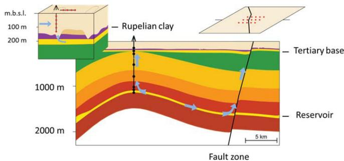
Fig. 10 Schematic of a geoelectrical monitoring concept for combined surface-downhole measurements being optimized for salinization detection at potential brine migration pathways [16]. Optimized electrode array designs, e.g. that penetrating the Rupelian clay barrier (indicated in purple), can provide monitoring beyond the particular CO<sub>2</sub> migration.
