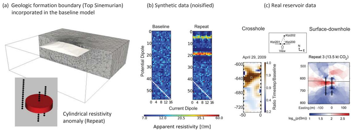
Fig. 3 (a) Synthetic geoelectrical modeling to investigate imaging characteristics and plausibility of field data; (b) The pseudosections show that only the electrodes in and near the reservoir are showing a time-lapse signal due to the migrating CO<sub>2</sub> (here: electrodes #4-#6 of Ktzi200 and electrodes #19-#21 of Ktzi201); (c) Real data results from a crosshole ERT inversion and SD-ERT inversion, which are found to be in reasonable agreement.
