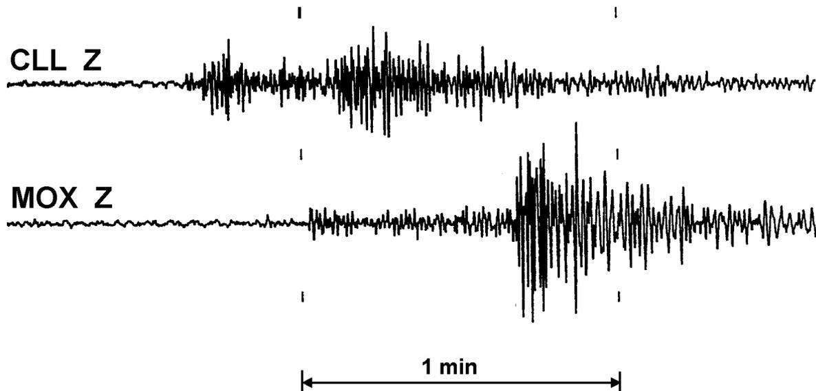
**Figure 1** Vertical component records of a local seismic event in Poland at the stations CLL and MOX in Germany at scale 1:1. The magnification values  $\text{Mag}(\text{SM})$  as a function of period  $T$  for this short-period seismograph are given in Table 1 below.
