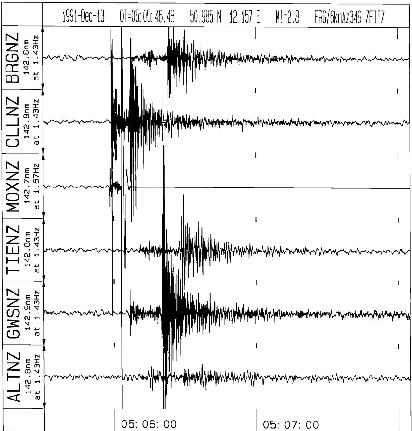
**Figure 2** Recordings of a near earthquake situated within the seismic network of stations shown in Figure 5. The time scale is 1 mm/s. Note the second strong onset in the record of station MOX has a very different form and frequency than in any other record. It is not a natural wave onset but a malfunction of the seismograph, which responds to the impulse of the strong Sg with its own impulse response.
