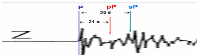
**Figure 7** Cutout of the vertical component record in Figure 2, stretched in time-scale. This allows better recognition of the depth phase onsets pP and sP at the expected arrival times after P for an earthquake at 111 km depth (as calculated by the ISC).
