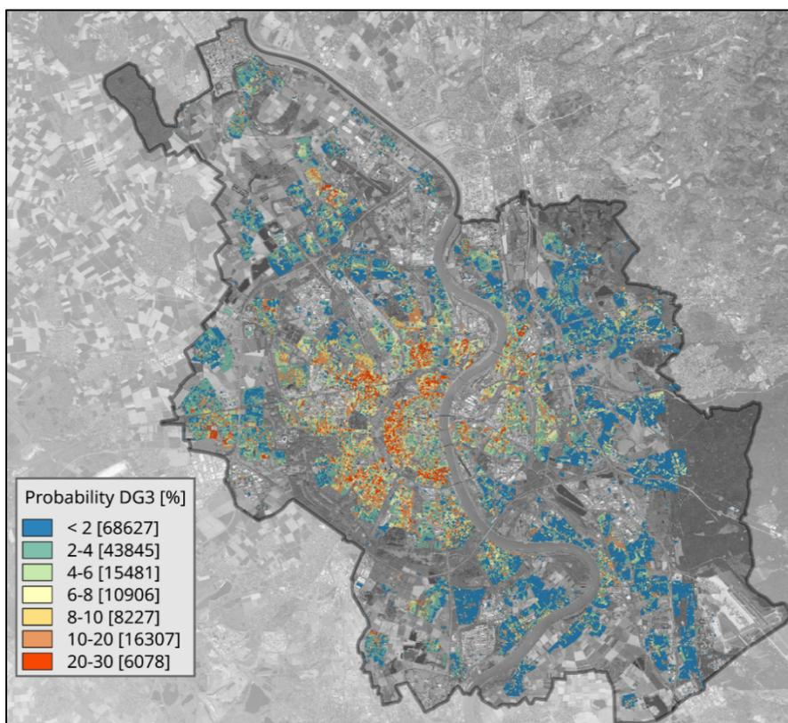
Figure 9.44: Probability of occurrence of damage grade 3 per building.
