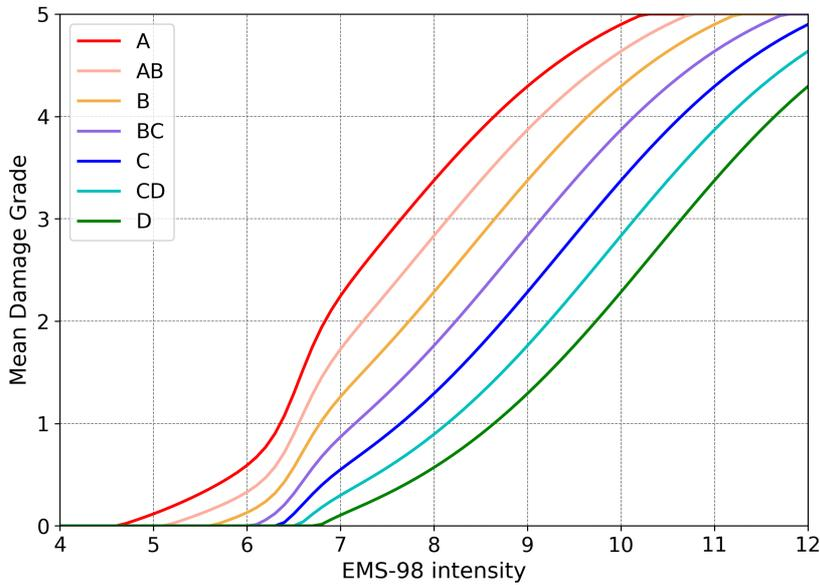
Figure 9.1: Mean damage grades for different EMS-98 vulnerability classes (color scale) and vulnerability indices C independent of number of stories.
