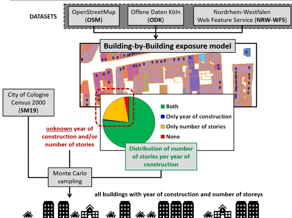
Figure 9.4: Schematic (simplified) representation of the process followed to generate the building exposure model for Cologne with year of construction and number of stories. An extensive description is given in the text.
