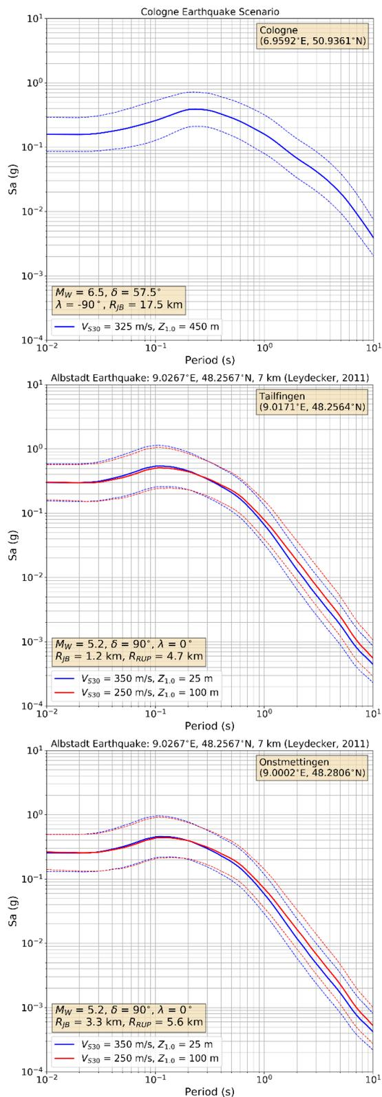
Figure 9.58: Response spectra for a site in the center of Cologne under the earthquake scenario studied herein (top) and for the center of the Albstadt districts of Tailfingen (center) and Onstmettingen (bottom) under a scenario reproducing the 1978 Mw 5.2 Albstadt earthquake calculated using the Boore et al. (2014) ground-motion model.
