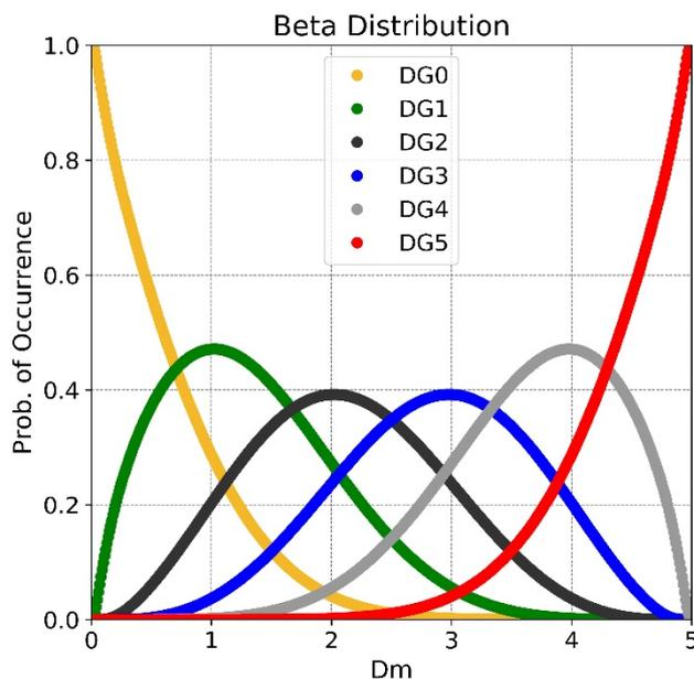
Figure 9.2: Probability of occurrence of each damage grade (color scale) as a function of the mean damage grade under the assumptions of a Beta distribution and the equivalences defined by Raschke (2003).
