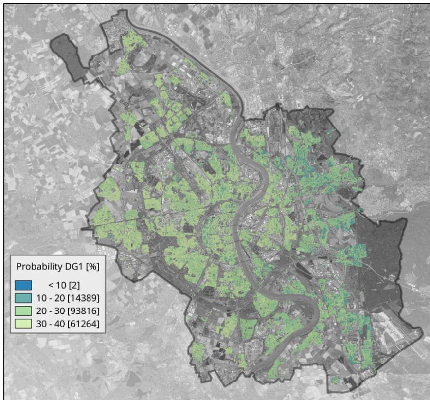
Figure 9.42: Probability of occurrence of damage grade 1 per building.
