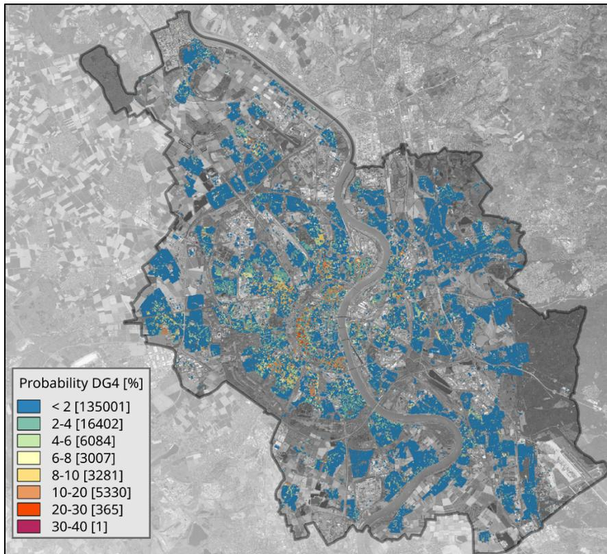
Figure 9.45: Probability of occurrence of damage grade 4 per building.
