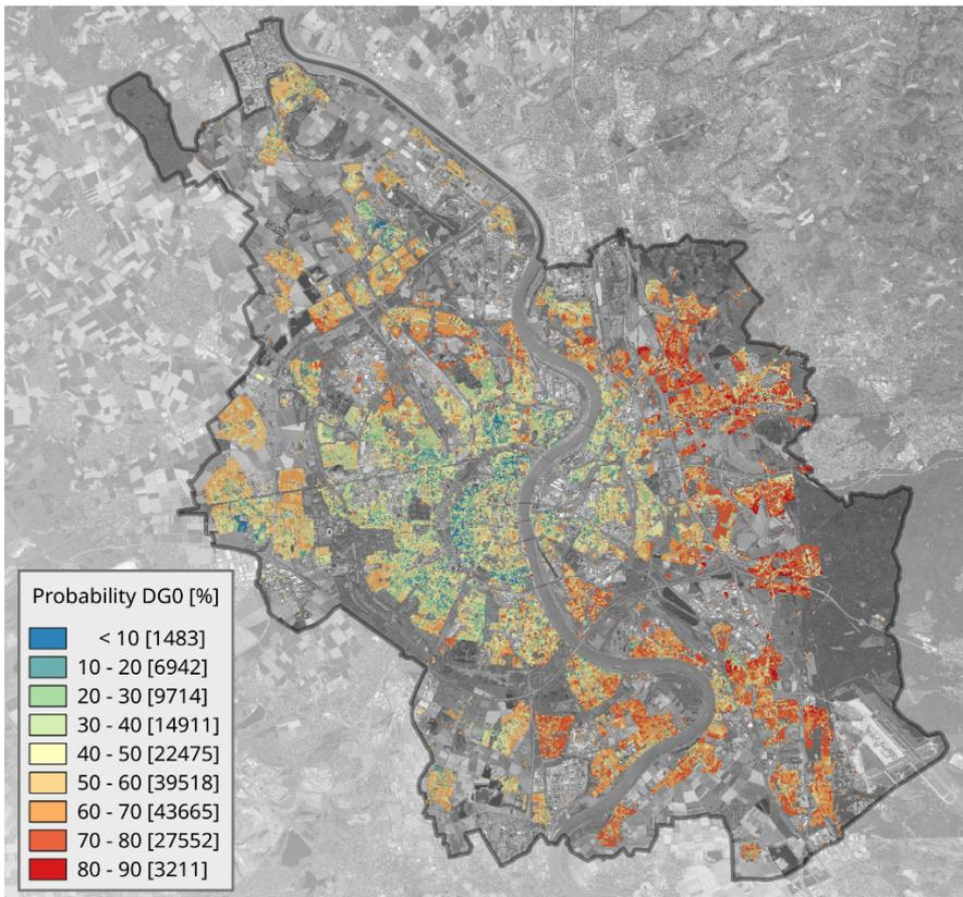
Figure 9.41: Probability of occurrence of damage grade 0 per building.
