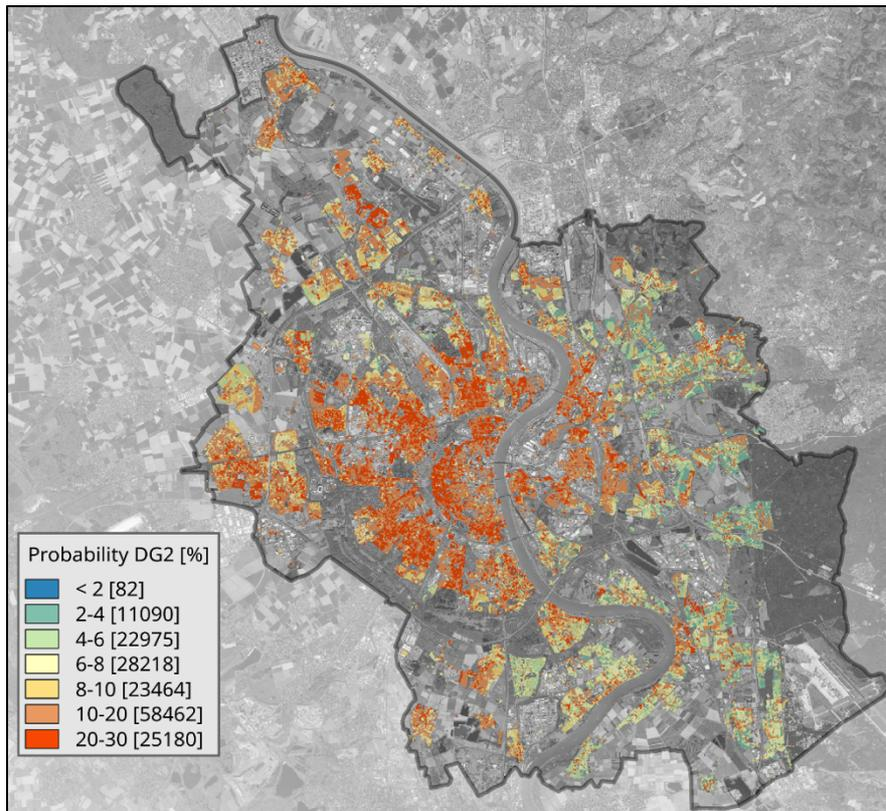
Figure 9.43: Probability of occurrence of damage grade 2 per building.
