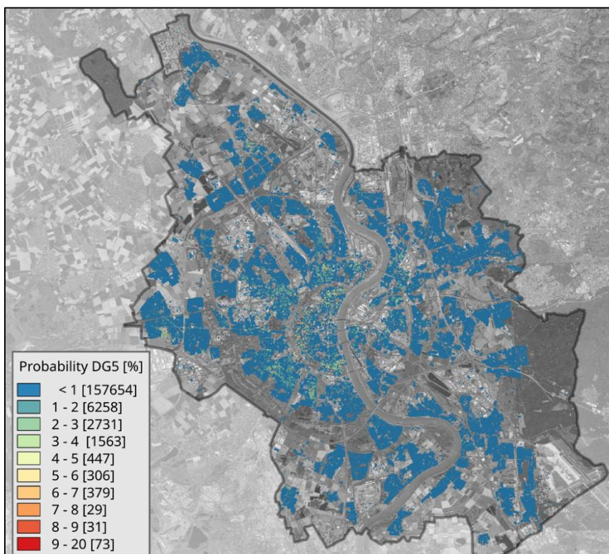
Figure 9.46: Probability of occurrence of damage grade 5 per building.
