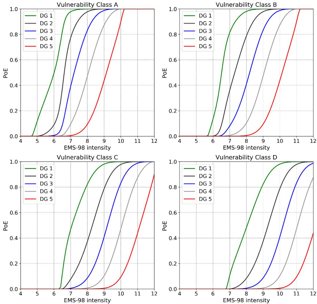
Figure 9.3. Probabilities of exceedance (PoE) of each EMS-98 damage grade resulting from the mean damage grade functions and the assumption of a Binomial distribution as described in the main text.
