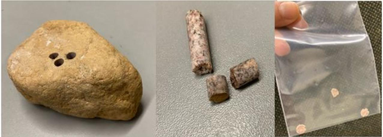
**Fig. 1:** Stepwise procedure of rock surface dating (one drilled metamorphic rock from the left, drill cores from the drilling process in the middle and very thin rock slices of ~0.8 mm thickness and ~7mm diameter at the right)
