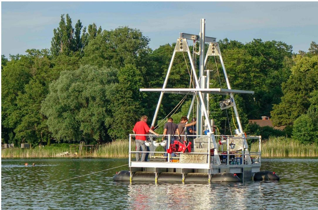
**Fig. 1:** UWITEC Niederreiter HYBRID 90 mm Piston Coring System operated on Groß Glienicker See in June 2020 (Foto: AWI)
