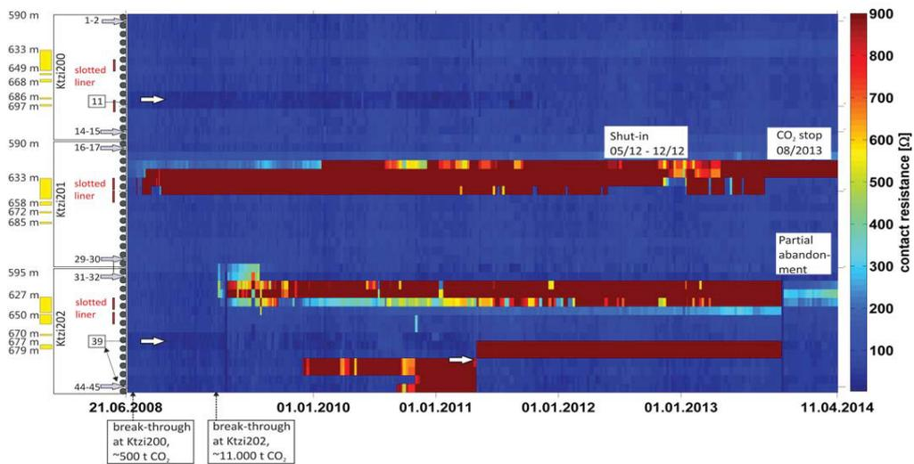
Figure 5: Update of the compact overview plot of contact resistances versus the injection history according [7], starting in June 2008 and ending in April 2014. In autumn 2013, the partial abandonment of Ktzi202 has caused as a side effect the sealing of the free annular space by overflowing cement suspension and subsequently better coupling of the electrodes along this section. The white arrows symbolize parts of the ERT arrays with gradually electrode degradation (#11, #39-#45).
